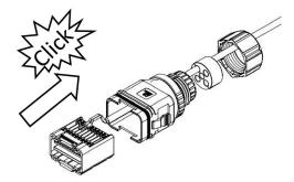
Install the plug into the main body and plug the holes without wires with a plug.
