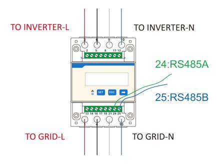
Insert L1/L2/L3/N wires and RS485A/B cable into the meter. Please refer to the meter wiring diagram on side of meter itself.
