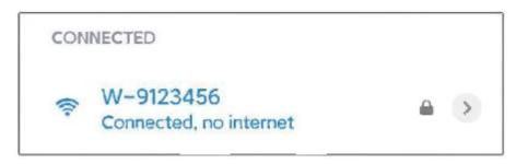
Step 2: After connecting successfully. Open browser and enter '192.168.1.1' on the address bar on top.
