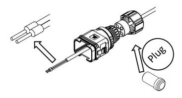
Insert the wires into the corresponding terminals.
