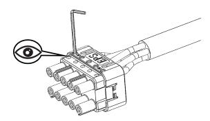
Insert the GRID end-core wire into the GRID end of the rubber core, observe the perspective hole cable in place, use S2.5 hex wrench to tighten the screws, torque  $2.5\pm0.1N\cdot m$ ;
