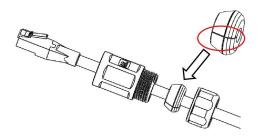
Stuck into the network cable through the gap on the sealing side.
