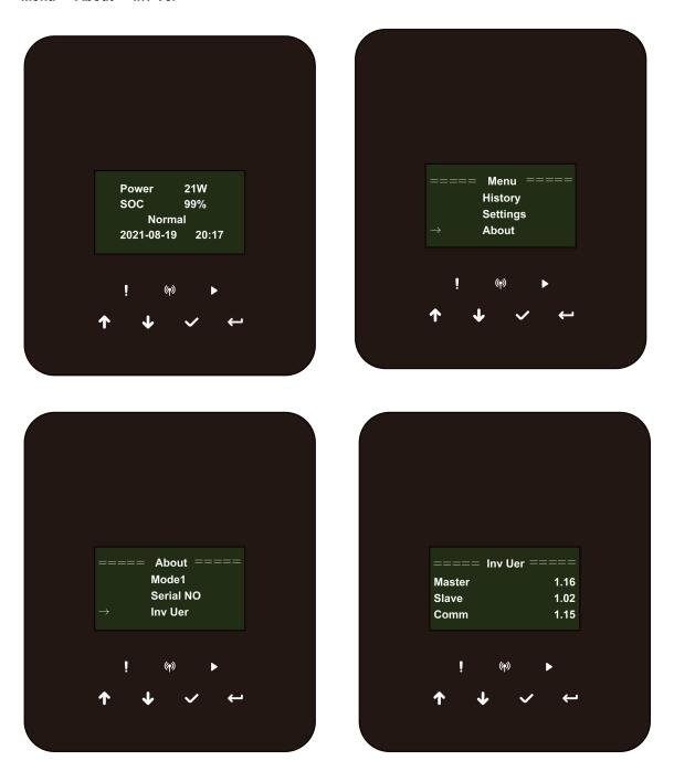
7. Turn on AC &DC breaker. If you updated the HMI, long press the "enter" and click "set" to turn on the inverter. Make sure the inverter can enter **Normal State**.
