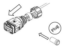
Lock wire nut screwed onto the body, torque 2.5+/-0.1N-m, then complete installation.
