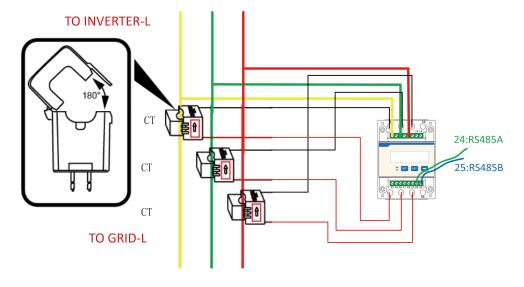
Notes: The 2,5,8 of the CT meter are connected to the three live wires L1, L2, and L3 respectively.
