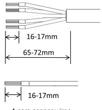
4-core copper wire+ Single-core copper wire
