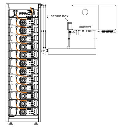
The P +\ P- terminal of the high-voltage box is connected to the P +\ P- terminal of the PCS
