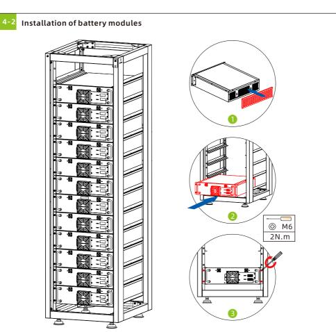
Install the battery modules into the slots of the rack from bottom to top.
