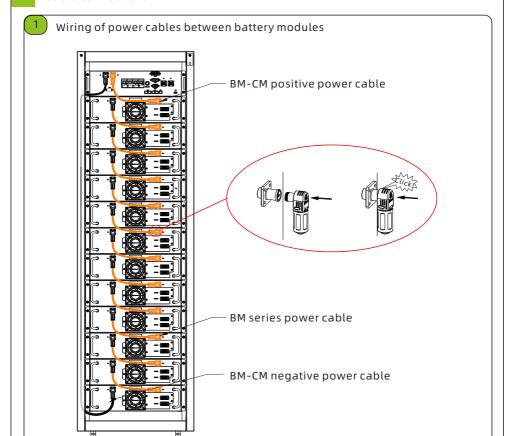
Please measure the voltage of each battery pack accurately before connecting the power cable. The bottom battery pack "B-" terminal is connected to the high-voltage box "B-" terminal. The "B+" terminal of the top battery pack is connected to the "B+" terminal of the high-voltage box.
